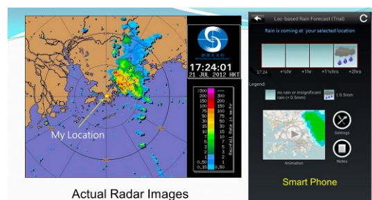
Figure 11. A comparison of the radar image with the location specific rainfall nowcast as shown on MyObservatory of HKO.
